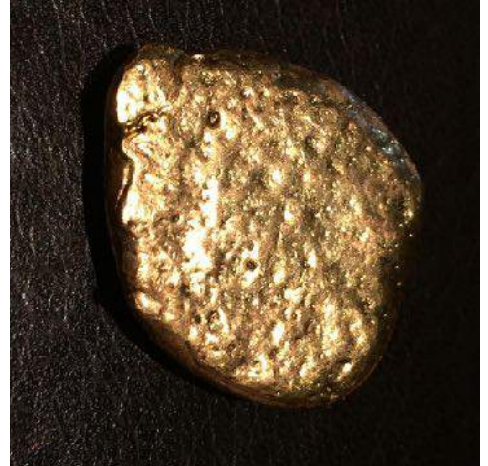
Gold Button from Metallurgical Testing
